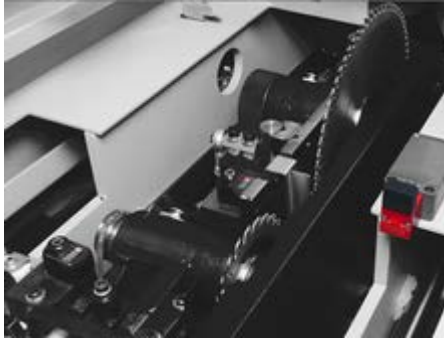
Saw carriage with main and scoring unit
