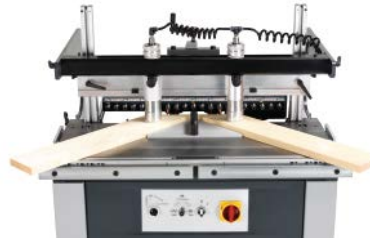
45° mitre fence for frame components
