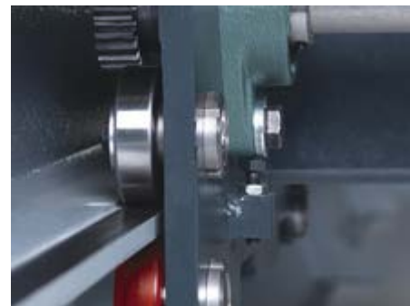
Double measuring system on the material pusher
