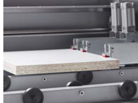
Pneumatically controlled, solid collet chucks made of steel
